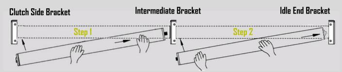
Step 1 Insert the "Metal Spindle Coupler" (spring idle side), then slide the clutch into the "Clutch Side Bracket".
