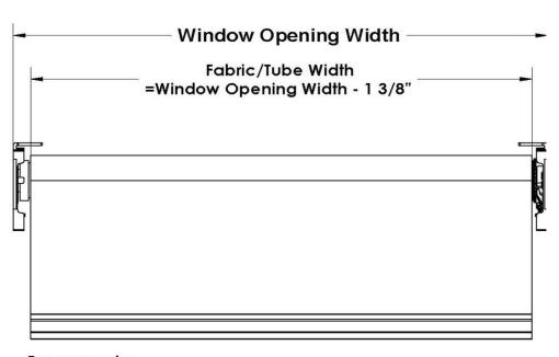
For example: Window opening width: 24" Fabric/Tube width: 22-5/8"
