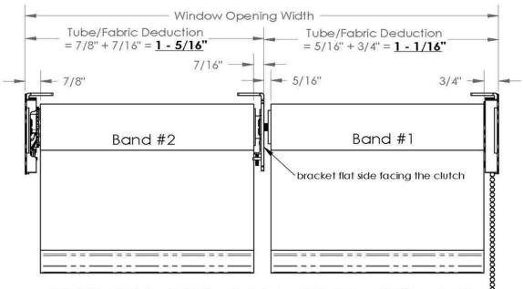
Total Tube/Fabric deduction for Intermediate Support(with end cap) = <u>1 - 5/16"</u> + 1 - 1/16" = 2 - 3/8"
