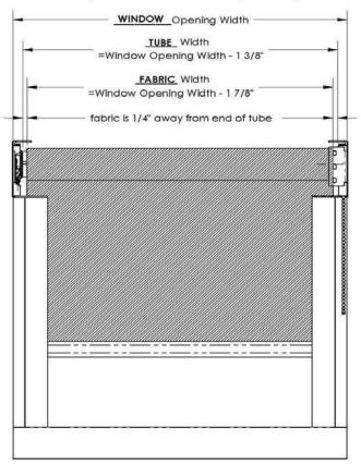
For example: Window opening width: 24" Tube width: 22-3/8"
