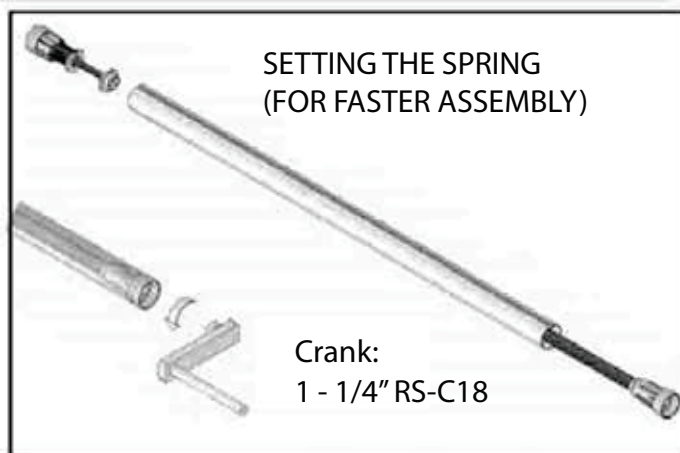
A - Use a crank to pre-load the spring in a clockwise direction
