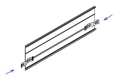
**2.** Hook 5.5" Fascia onto the mounted 5.5" Smart Head Box Brackets.
