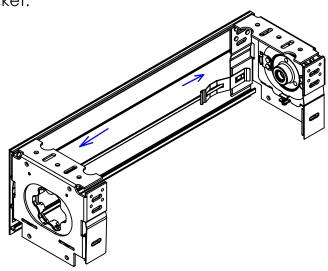
**4.** After 5.5" Fascia is fixed on the both sides brackets, hang on the Bottom Closure Panel to 5.5" Fascia.
