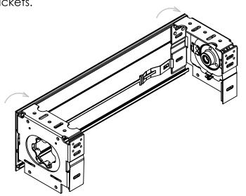
**3.** Slide a Spring Lock towards drive side bracket and locks with it; Operate the same way at the idler side bracket.
