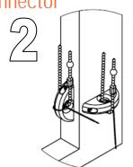
Place tensioner on the wall where the bead chain can be taut but allow the connector or stopper to go through smoothly
