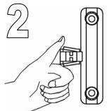
Insert "plug" into shell to close the gap. Make sure it fully snaps in. Position tensioner onto the wall then follow steps 3 and 4 as above.
