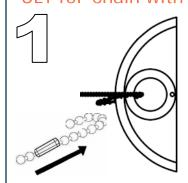
Insert bead chain into the hole then position tensioner vertically (for inside mount) or horizontally (for outside mount).
